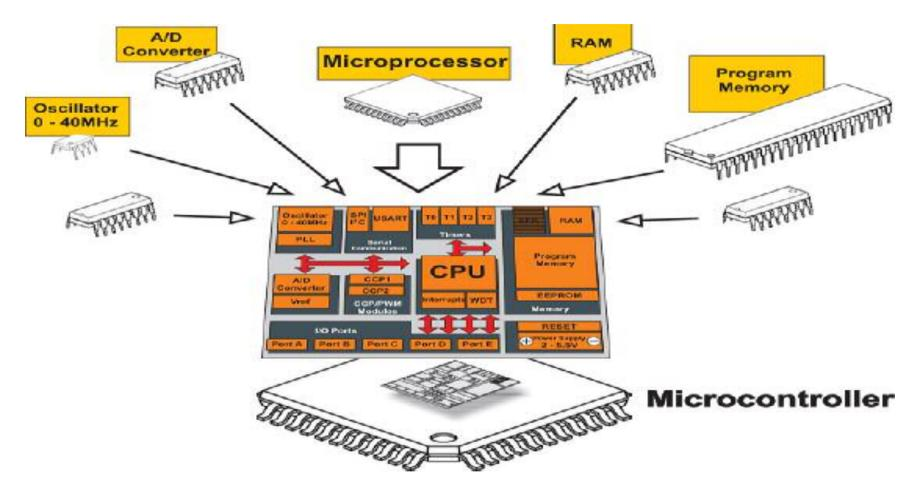
The MC is designed to be all of that in one. No other external components are needed for its application because all necessary circuits belong to peripherals are already built in it. It saves time and space needed to design a device.
