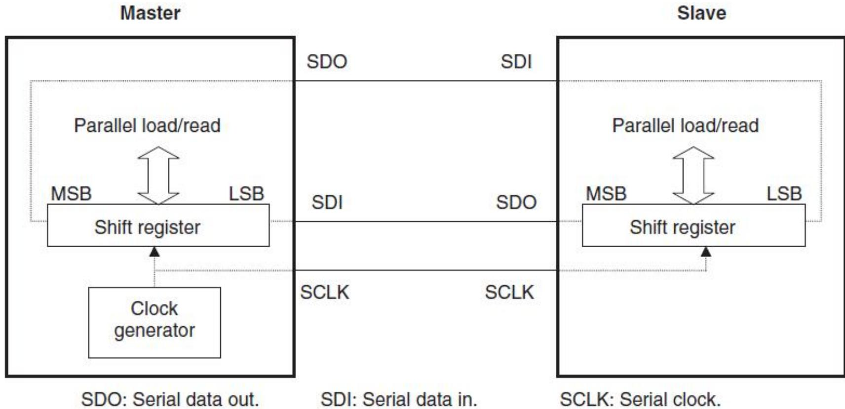
The synchronous serial link implemented in a microcontroller
