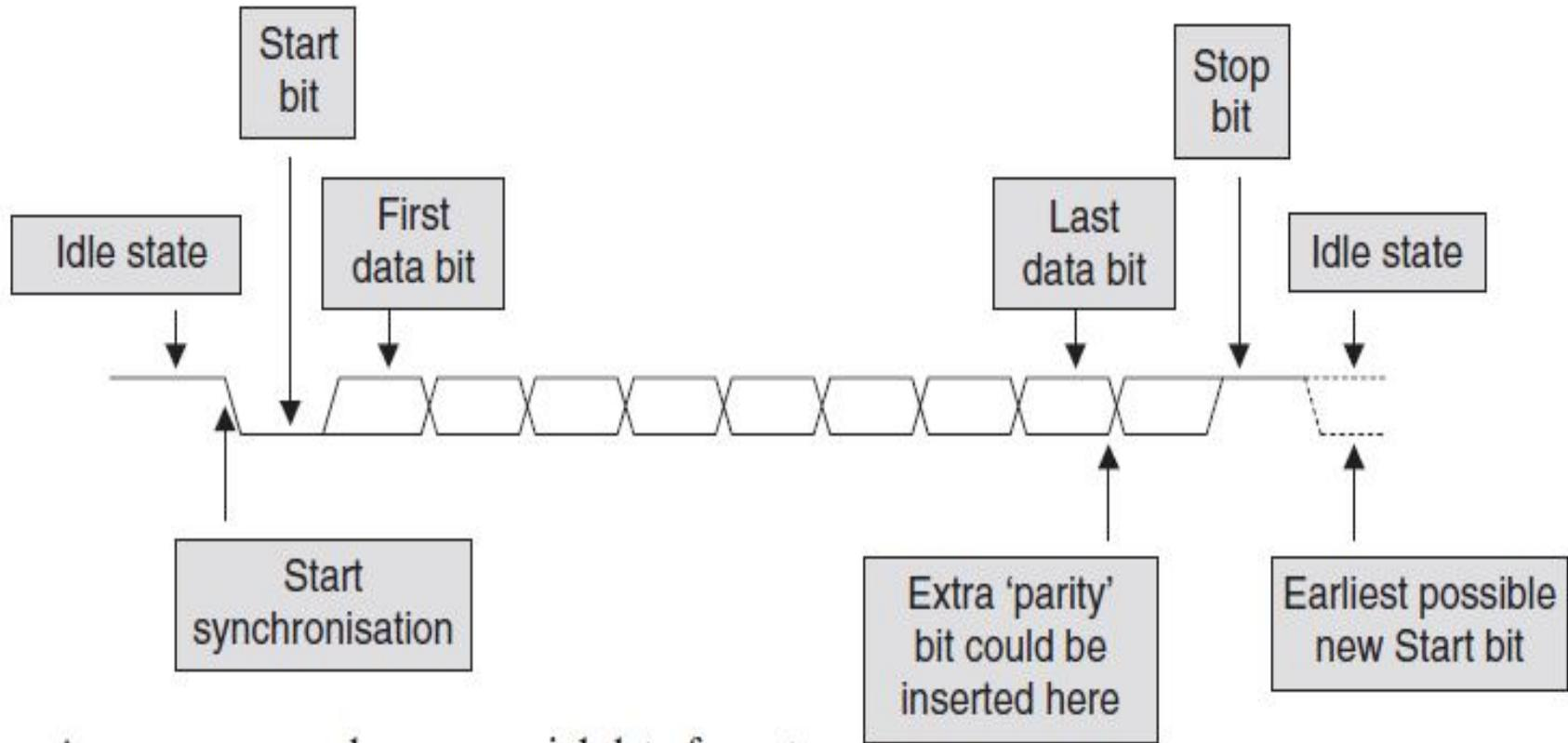
A common asynchronous serial data format
