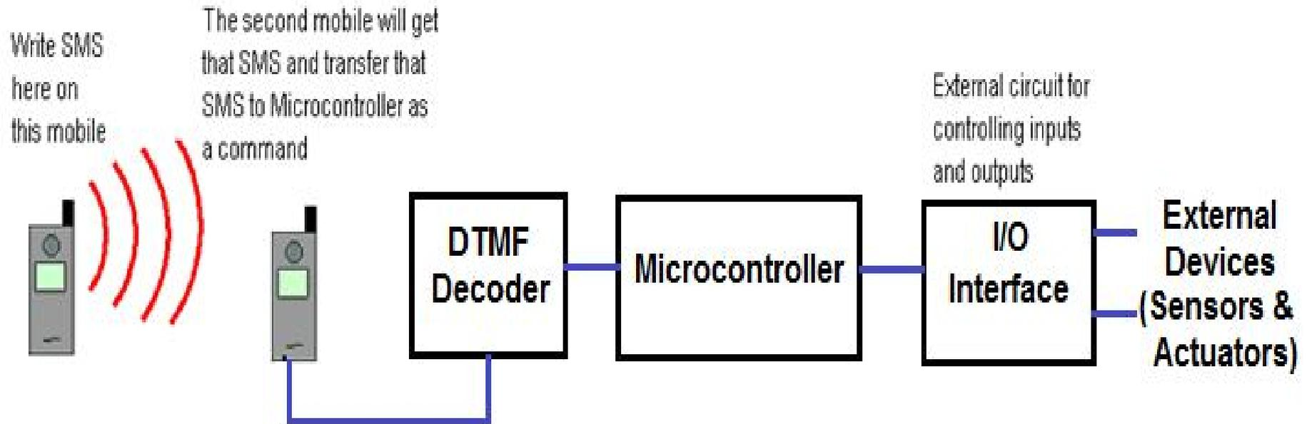
The MT8870D/MT8870D-1 is a complete DTMF receiver integrating both the bandsplit filter and digital decoder functions. The filter section uses switched capacitor techniques for high and low group filters; the decoder uses digital counting techniques to detect and decode all 16 DTMF tone-pairs into a 4-bit code.
