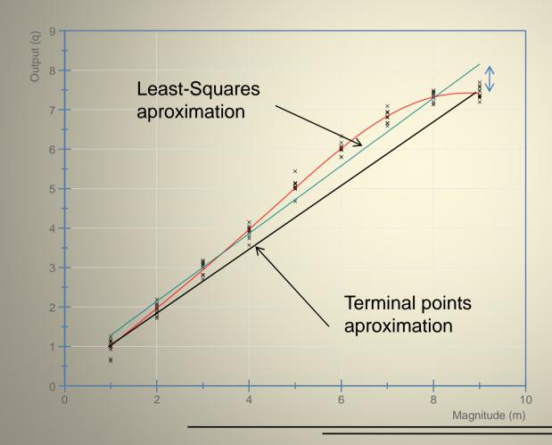
•Associated to a linear approximation of the transfer function.
