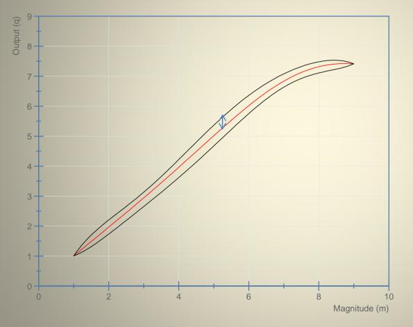
•Deviation of the sensor's output at specified point when it is approached from the opposite directions (usually in percent of FS value)
