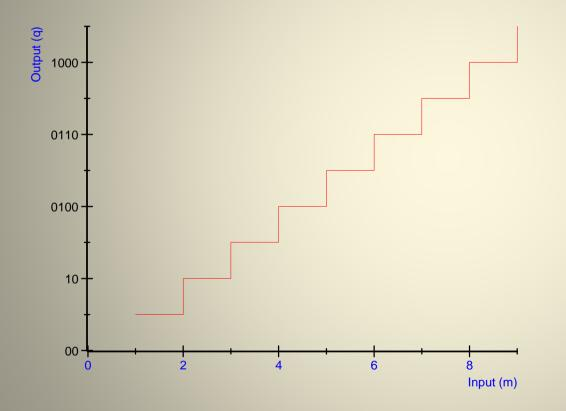
• In sensors with discrete response (after ADC conversion for exampled), the minimum resolution achievable is usually limited by A/D quantization error (step size).
