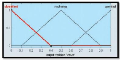
Write **MATLAB Program** to construct an FIS system using **Mamdani** method with the following properties: **AndMethod = min, OrMethod = max, ImpMethod = min, AggMethod = max, DefuzzMethod = centroid Evaluate** the output of a fuzzy system for a given input (**0.8**).
