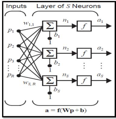
• The units can be distinguished as input units, which receive signals from the outside world, and output units, from which the response of the net can be read. A one-layer network, with **R** input elements and **S** neurons, is shown below. In this network:
