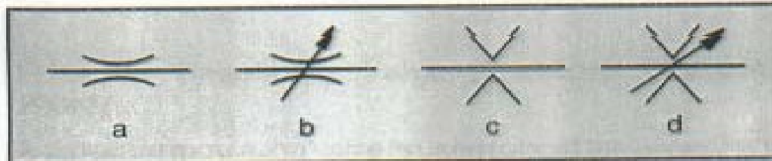
Graphic symbol acc. to DIN ISO 1219 a) Throttle, fixed, b) Throttle adjustable, c) Disc throttle, fixed, d) Disc throttle, adjustable
