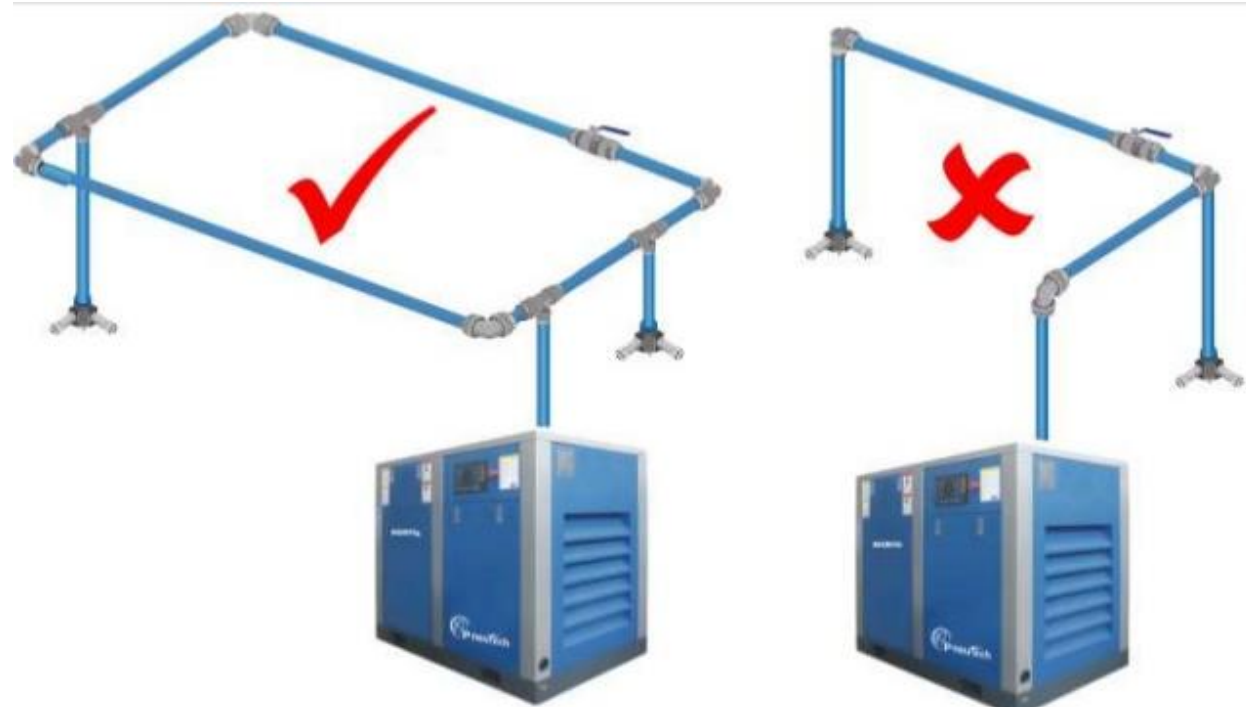
Correct Ring Main System for consistent air flow and pressure to all outlets
