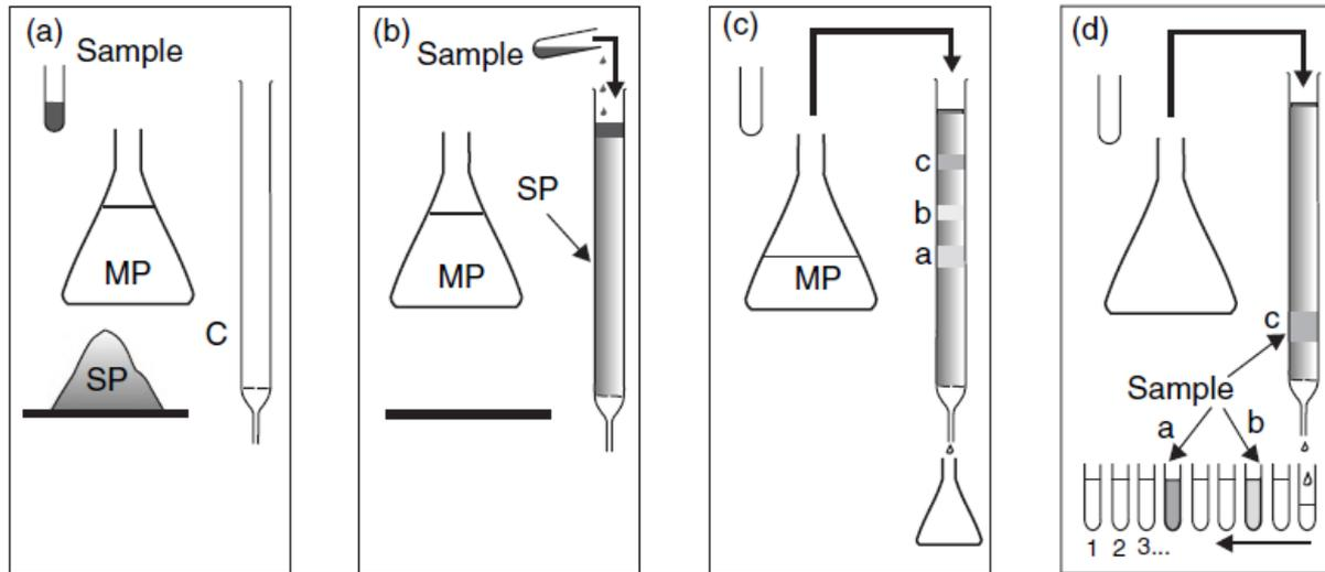
**Figure 1.1** *A basic experiment in chromatography.* (a) The necessary ingredients (C, column; SP, stationary phase; MP, mobile phase; and S, sample); (b) introduction of the sample; (c) start of elution; (d) recovery of the products following separation.
