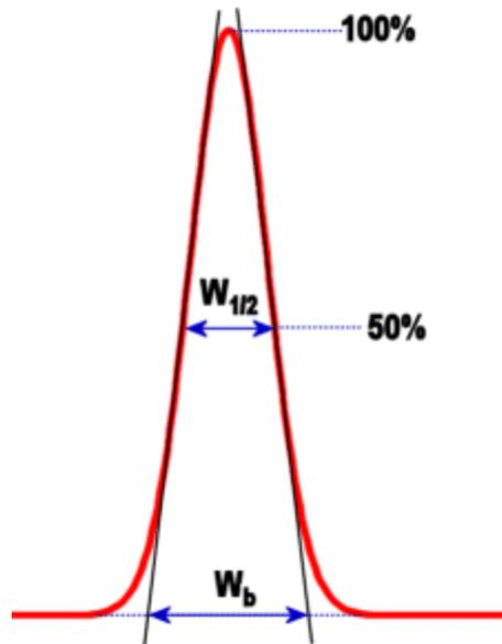
**Baseline width ( $W_b$ ).** This is measured by drawing tangents to the front and back slopes of the peak. The baseline width is the distance between the intersections of these tangents with the baseline.
