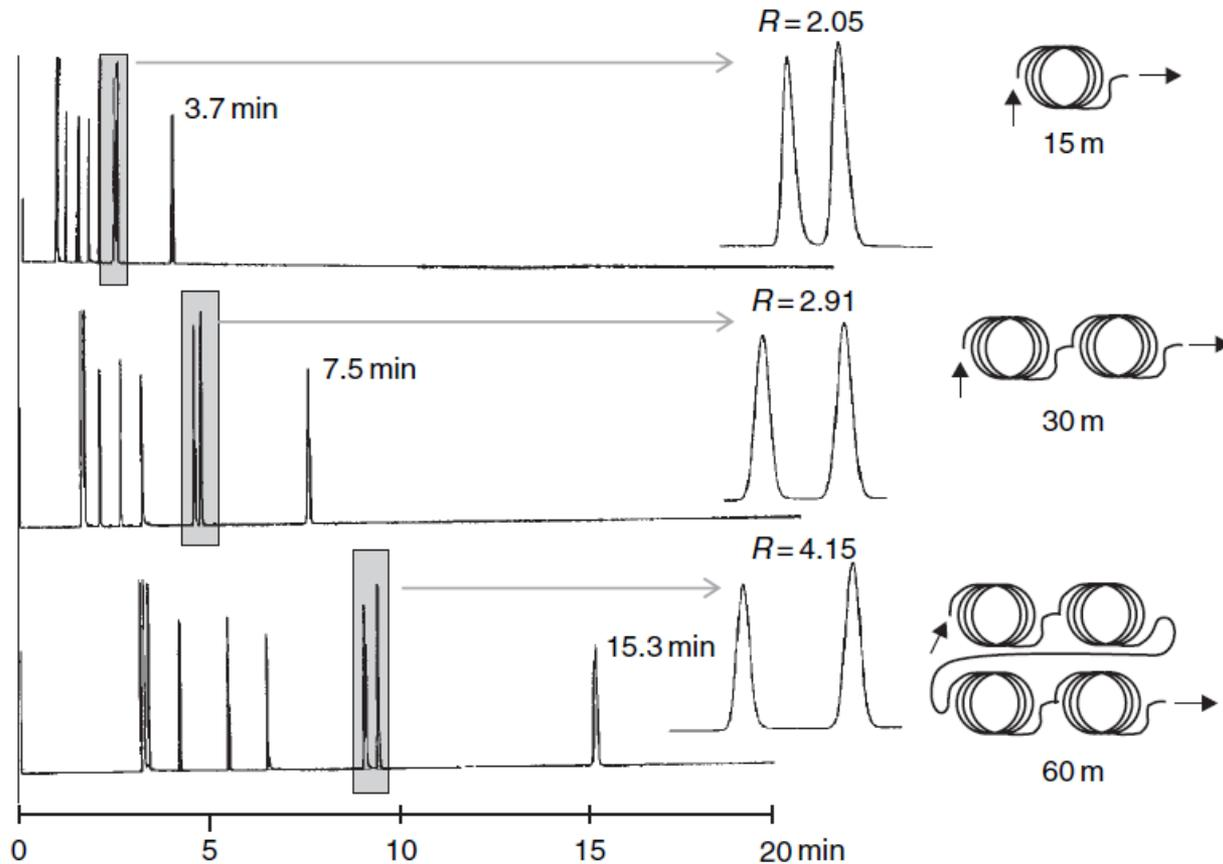
Q. How are the  $R$ ,  $H$ ,  $k$ ,  $K$ ,  $t_R$ ,  $t_m$ ,  $t_R'$ , and  $\alpha$  will be affected by doubling the column length?
