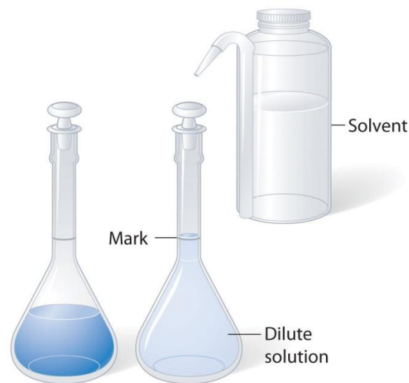
(c) The measured volume in the second flask is then diluted with solvent up to the volumetric mark [(V_s)(M_s) = (V_d)(M_d)] .
