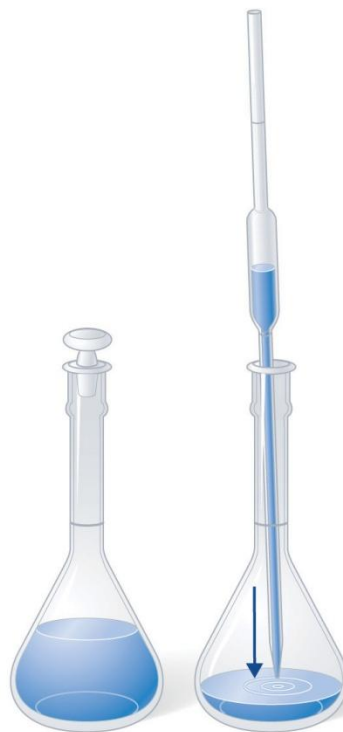
(b) The measured volume of stock solution is transferred to a second volumetric flask.
