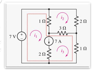
**Example 4:** Determine the three mesh currents in the shown figure.
