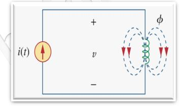
Any change in  $\phi$  is caused by a change in the current.
