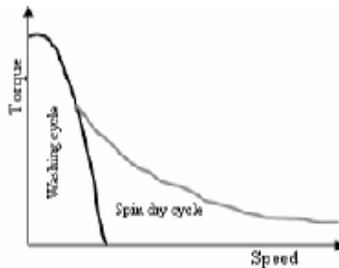
Fig. 1. Typical torque-speed characteristic of direct drive washing machines.
