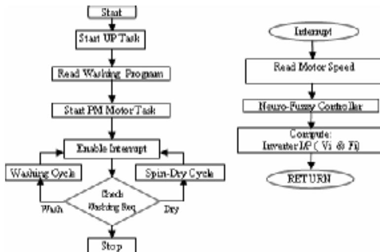
Fig.7. Real-time software design.
