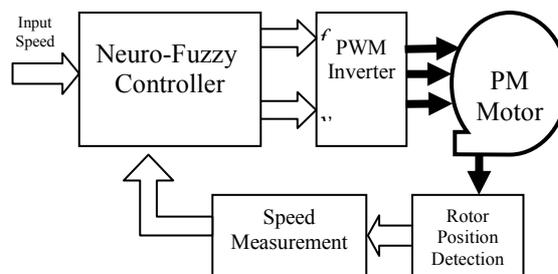
Fig. 4. Sensorless PM Motor drive system.
