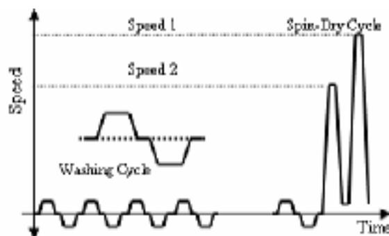
Fig. 2. Cycles of direct drive washing machines.
