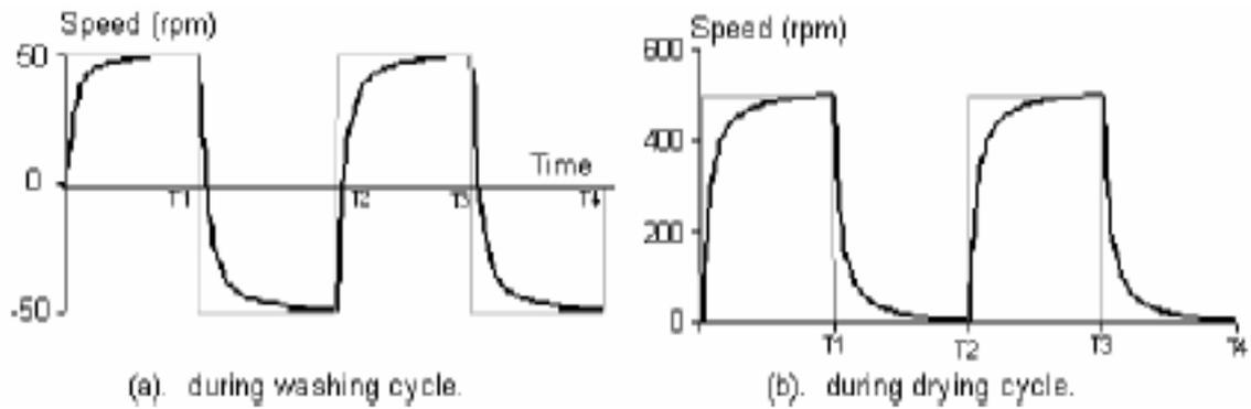
Fig.10. Transient response during washing and drying cycles.
