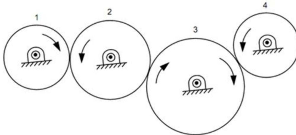
□ When gears are meshed in gear train, one of the gears is **drive** (input) and the others are **driven**. However, one of the driven gears is called **output**
