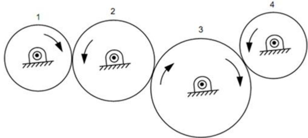
$$\frac{\omega_4}{\omega_1} = -\frac{\omega_2}{\omega_1} \times -\frac{\omega_3}{\omega_2} \times -\frac{\omega_4}{\omega_3} = -\frac{N_1}{N_2} \times \frac{N_2}{N_3} \times -\frac{N_3}{N_4} = -\frac{N_1}{N_4}$$
