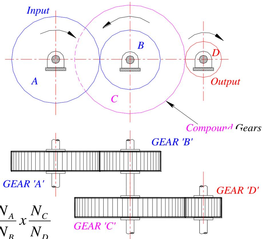
$$\frac{\omega_D}{\omega_A} = -\frac{\omega_B}{\omega_A} \times \frac{\omega_C}{\omega_B} \times -\frac{\omega_D}{\omega_C} = \frac{\omega_B}{\omega_A} \times \frac{\omega_D}{\omega_C} = \frac{N_A}{N_B} \times \frac{N_C}{N_D}$$
