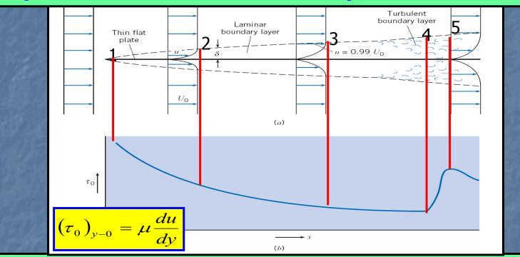
The boundary layer thickness is very thin, occurs because of the viscosity of the fluid.
