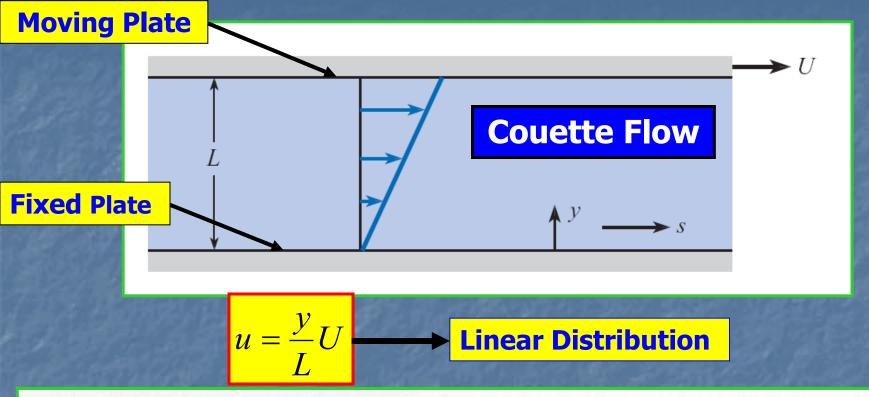
which shows that the velocity profile is linear between the two plates. The shear stress is constant and equal to
