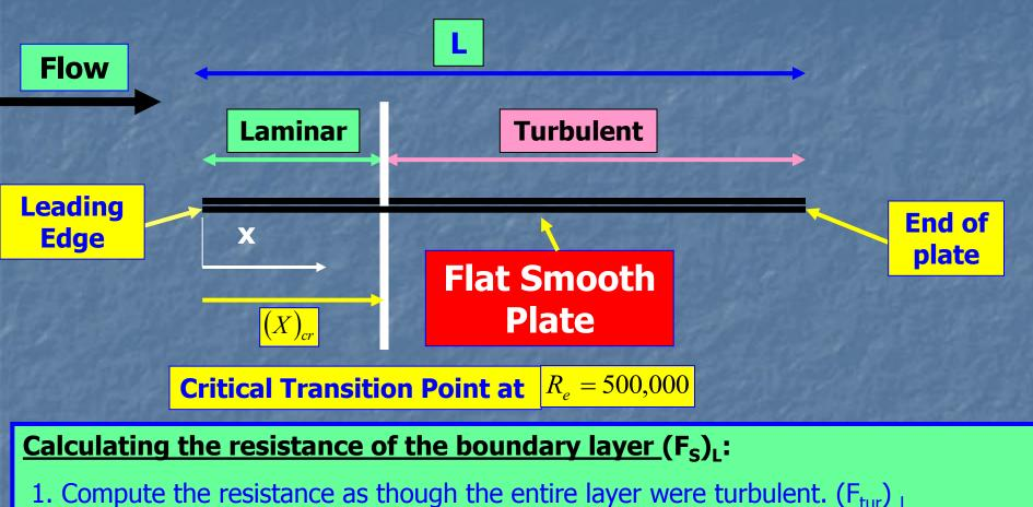
2. Compute the resistance of the laminar part,  $(F_{lam})_{Ltr}$  and the resistance of the
