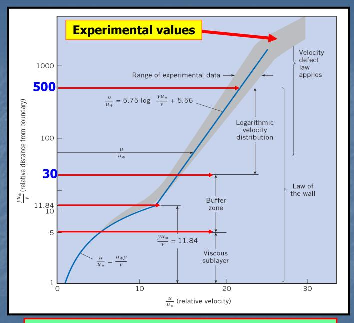
Velocity distribution in a turbulent boundary layer
