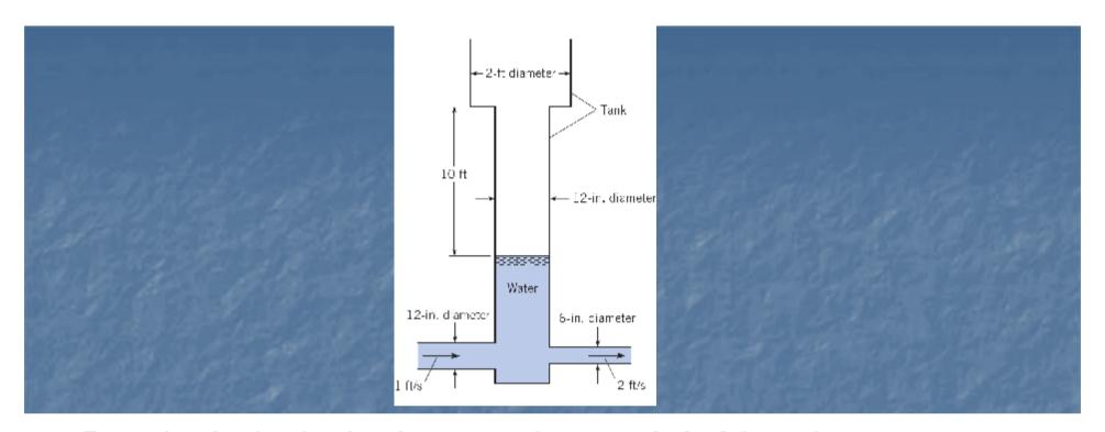
Determine the time it takes the water surface to reach the 2 ft. section:
