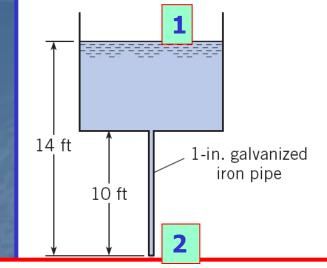
Situation: Water drains from a tank through a galvanized iron pipe. D = 1 in. Total elevation change is 14 ft. Pipe length = 10 ft.
