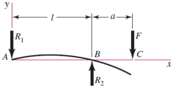
$$R_1 = \frac{Fa}{l} \quad R_2 = \frac{F}{l}(l + a)$$
