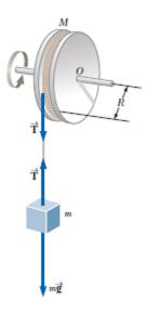
A disk of mass  $M=0.2\ kg$  and radius  $R=5\ cm$  is attached coaxially to the massless shaft of an electric motor. The motor runs steadily at  $900\ rpm$  and delivers  $2\ hp$ .
