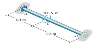
$T_A + T_B - 300 = 0$  $\phi_{C/A} = \phi_{C/B}$  $\frac{T_A(0.4)}{JG} = \frac{T_B(0.8)}{JG}$  $T_A = 2.00T_B$
