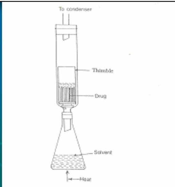
Apparatus For Continuous Extraction Of Drugs
