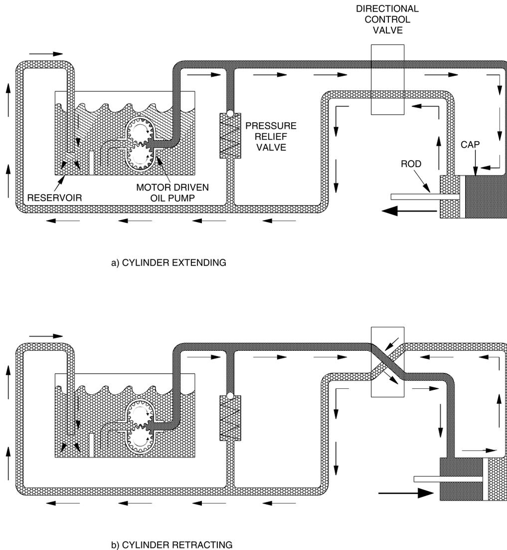
**Figure 1-4. Basic hydraulic circuit.**
