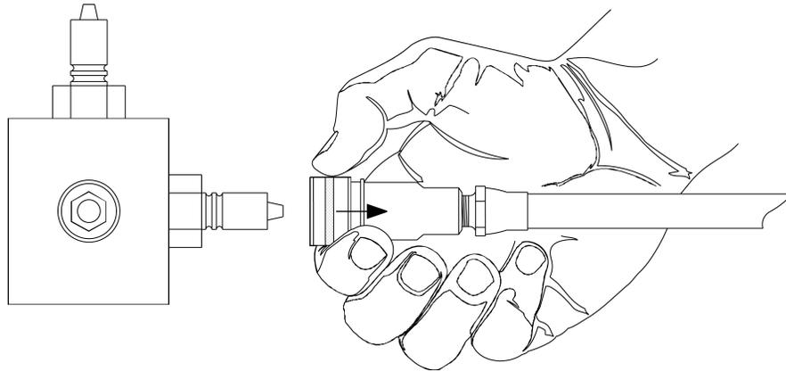
**Figure 1-15. Connecting and disconnecting a hose.**
