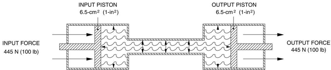
Figure 1-2. Direct transfer of force.
