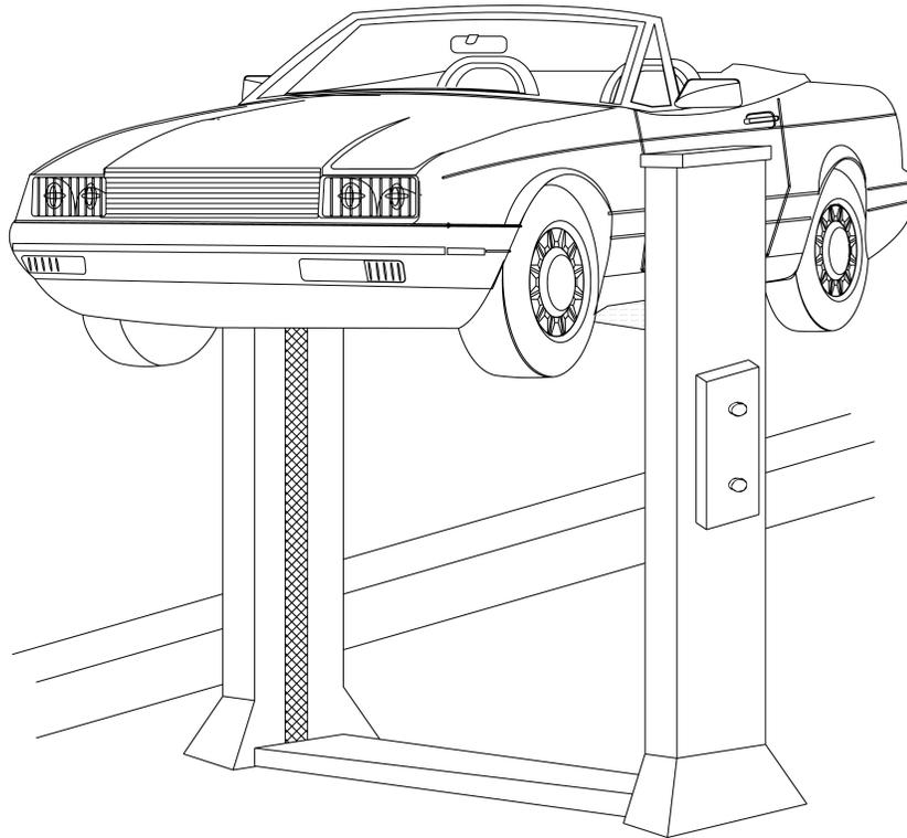
Figure 1-1. Hydraulic hoist.
