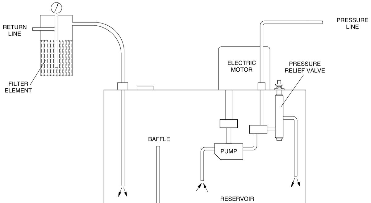
Figure 1-7. Inside view of the Power Unit.
