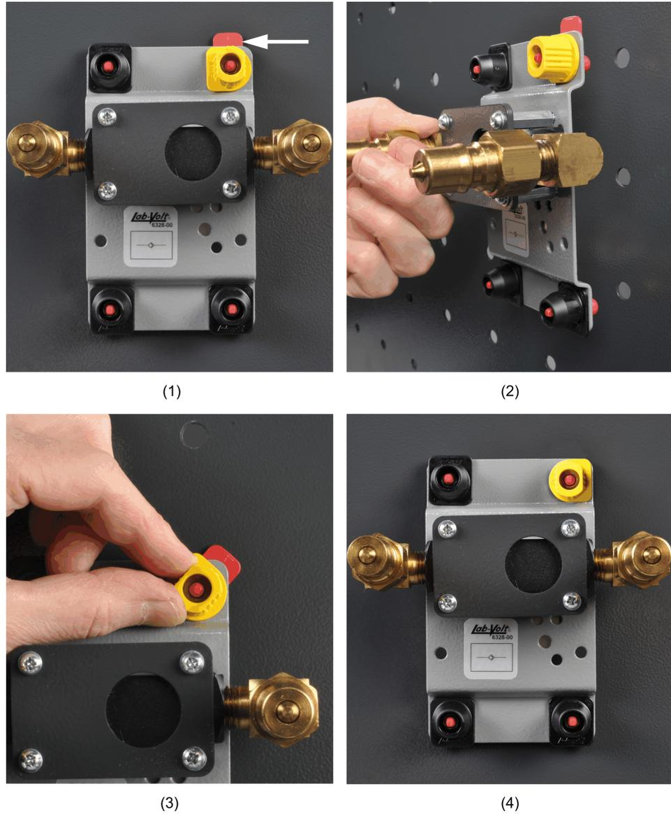
Figure 1-5b. Securing a component to the work surface with the Quick-Lock System.
