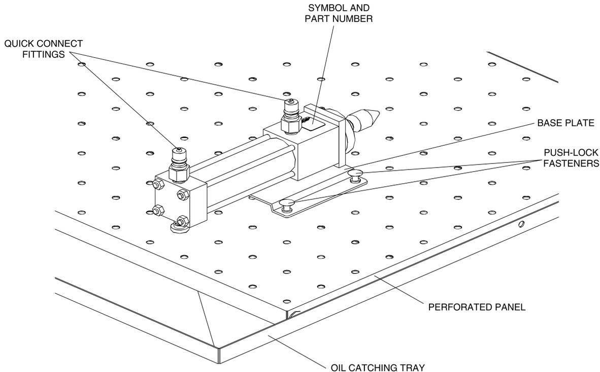
Figure 1-5a. Securing a component to the work surface with push-lock fasteners.
