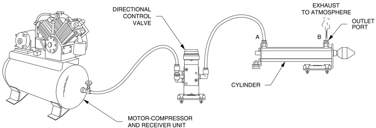
Figure 1-18. Fundamental Circuit Flow.
